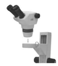
Warning: Do not tighten the screw too tight as this will cause damage to the instrument.
