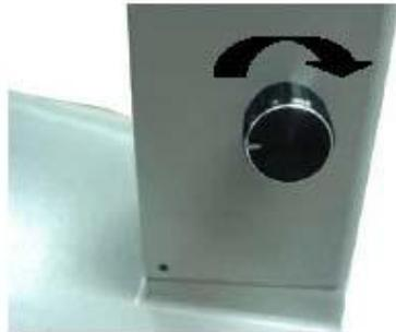
★ Adjust the black knob at the right side of column for the brightness of bed light source, attaining the sharp image outline. The arrowhead direction is the rotating direction for increasing brightness. The reverse direction is for brightness attenuating and turning off the bed light source power.
