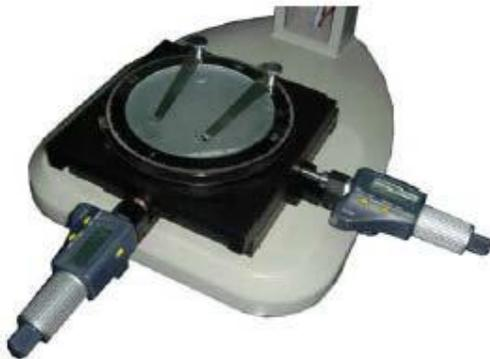
★ Install another micrometer in the same way and steps to the movable platform clamp spring. Tighten the fastening screw to clamp the support rod of micrometer to the extent of not shedding off and not rotating. Put it into the black/white workbench or single sided frosted glass workbench (note that the smooth surface should be facing upward). The final installation structure is as shown in the diagram.
