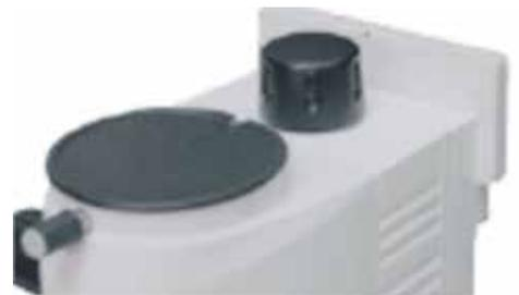
Photo above shows microscope light intensity control.
