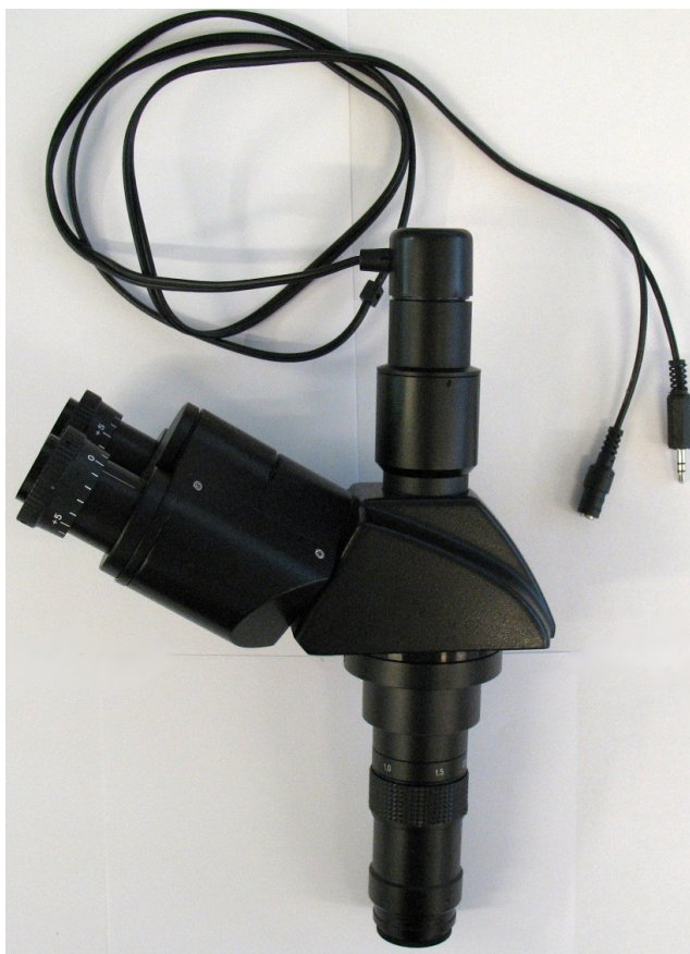
4 - OPTICAL HEAD WITH BUILT-IN DIGITAL CAMERA
