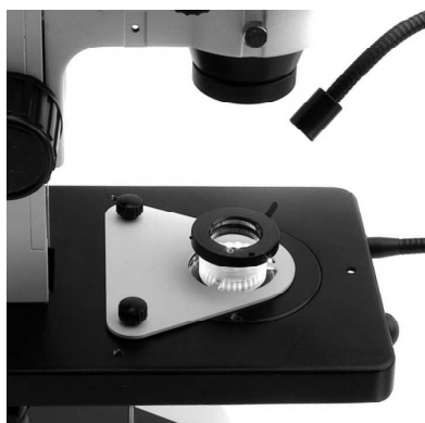
FIG. 6: IRIS APERTURE DIAPHRAGM FOR DARK FIELD USE
