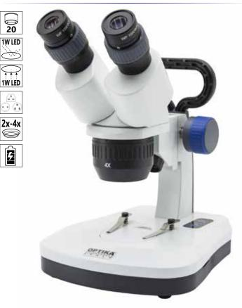
Binocular stereomicroscope equipped with turnable objective (2x-4x), fixed arm with handle, and incredibly bright and uniform led illumination (transmitted and incident), settable through the exclusive touch control. Powered by rechargeable batteries.
