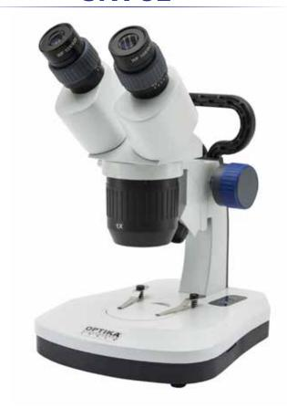
Binocular stereomicroscope equipped with turnable objective (1x-3x), 360° rotating head, fixed arm with handle, and incredibly bright and uniform led illumination (transmitted and incident), settable through the exclusive touch control. Powered by rechargeable batteries.
