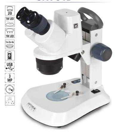
Digital binocular stereomicroscope equipped with with 3 magnifications turnable objective (1x-2x-4x), precision fixed arm with handle, and incredibly bright and uniform led illumination (transmitted and incident), settable through the exclusive touch control. Powered by rechargeable batteries.
