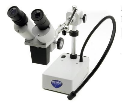
Binocular stereomicroscope equipped with fixed objective (2x), swiveling LED incident illumination on an overhanging, flexible arm. Ideal for long working distance (119 mm with standard 2x objective, 165 mm with ST-025, 124 mm with ST-026).
