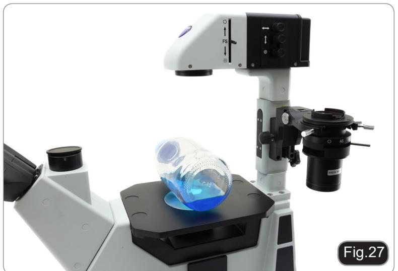
Once terminated the observation return the illumination column to its original position and lock the knob.
