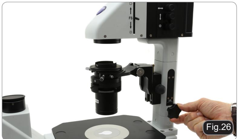
Rotate the knob on the right side of the illumination pillar (Fig. 26) to unlock the rotation, then swing out the condenser holder from the light path (Fig. 27).
