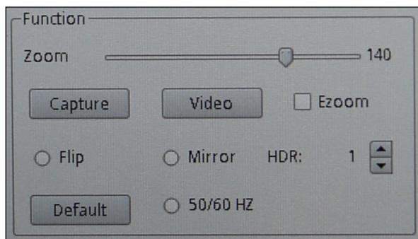
The “**Zoom**” cursor allows to vary the magnification of the projection to the monitor of the framed object.
