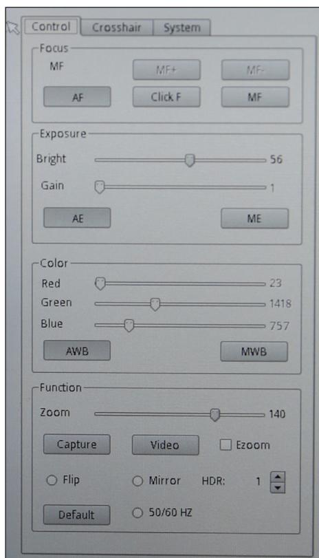
The “Control” panel is divided into different sections related to the various camera controls.
