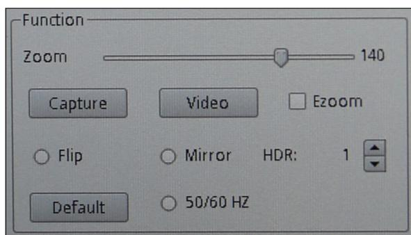
The variation of the electronic zoom factor will occur only and exclusively acting on the buttons at the bottom right of the monitor.
