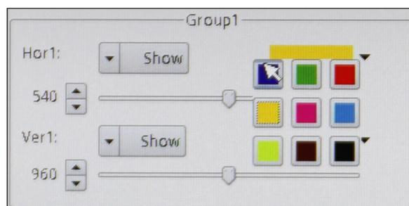
The lines, once traced, can be visible or hidden. Clicking on the “**Show / Hide**” button opens the context menu with which you can view a “**Show**” row or hide it “**Hide**”. The lines, if hidden, will not be deleted from memory but simply will not be visible.
