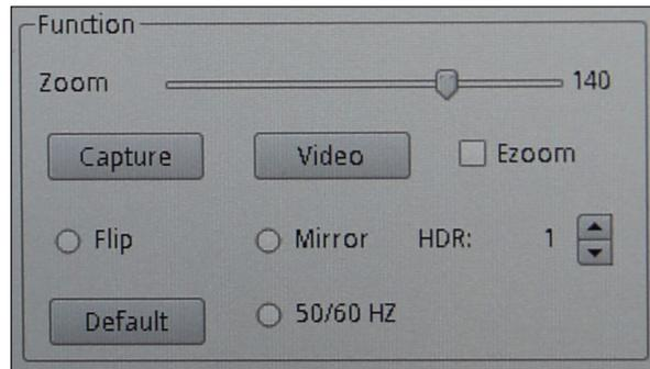
An **"HDR"** setting of 0 indicates that the camera will acquire a single image and store it. Increasing the number (max 3) the camera acquires 3 images at different exposures (usually an underexposure, one with optimal exposure and one overexposed), combines them to optimize the different zones with different lighting and creates a single image at exposure "virtually correct."
