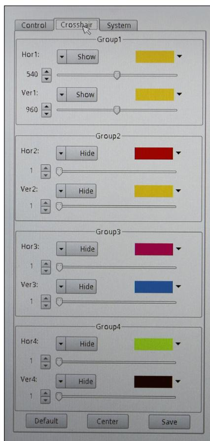
Up to 4 sets of horizontal or vertical rows can be superimposed on the monitor.
