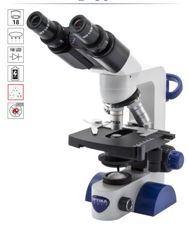
Cordless, modern binocular microscope ideal for students and mainly primary schools with achromatic lenses (400x), FN 18 eyepieces, finite optical system, coaxial focusing, StagErase™ eraseable mechanical stage, Abbe condenser and 1 W LED illumination with rechargeable batteries. Slim and easy to carry, it is equipped with arm/wrist rest support to reduce the fatigue during use and long lasting LED illumination to provide over 20 years of use
