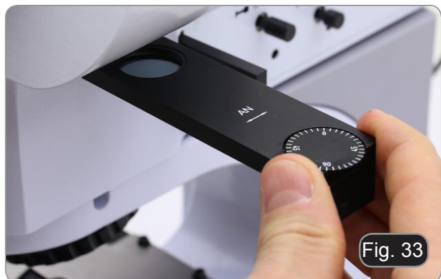
3. Put a flat mirror on the stage and get into approximate focus the mirror surface.
