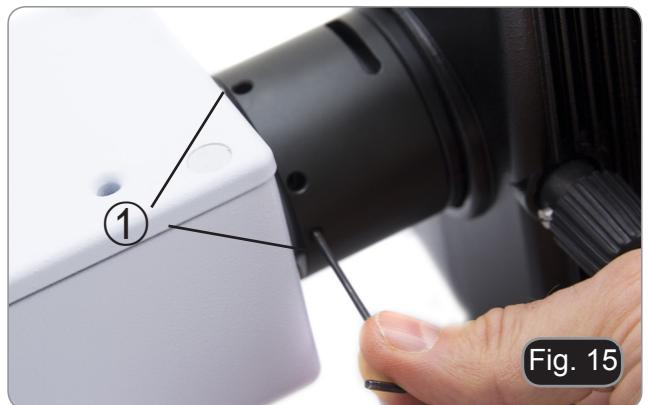
2. Insert the lamp housing extension tube and tighten the screws ②. (Fig. 16)
