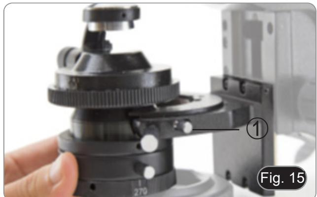
8. Mount the rotating stage: at the bottom of the stage there is a spring, push this spring toward the stage support ①, then push the stage downward ②. (Fig. 16)
