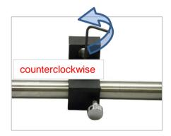
If drive unit of manipulator sway toward of back, turn the screw to the counterclockwise direction and push the drive unit of manipulator.
