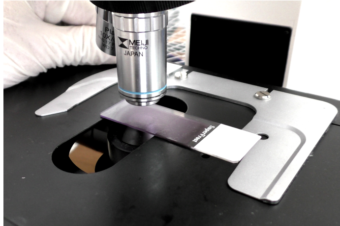
Fig. 5. Placing a slide on the microscope stage
