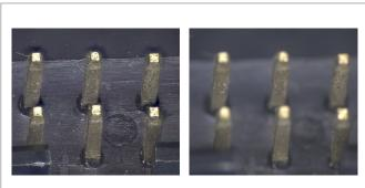
The clear images obtained through real-time depth of field fusion
