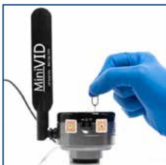
**Note:** MiniVID WiFi operates at 5GHz frequency for maximum speed (frames per second). If you need camera to operate at 2.4GHz on an older device that is not 5GHz compatible, use the included pin to press the Reset button for 1 to 2 seconds (camera frame rate will be slower than 5GHz speed). Repeat process to return to 5GHz speed.
