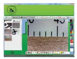
2 Put the d-VID microscope on the Calibration Pattern sheet, you can see the black/white block on the screen.
