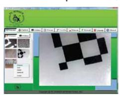
1 Click Calibration icon  $\oplus$ , and set the magnification to 50x for standard magnification.
