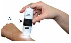
4 The zoom will be larger as d-VID digital microscope is closer to the observed object.
