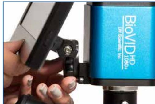
Remove the monitor from its packaging and mount the monitor to the camera's front mounting bracket using the included thumbscrew. Do not overtighten the thumbscrew but ensure you securely tighten it to prevent the monitor from falling off of the camera.
