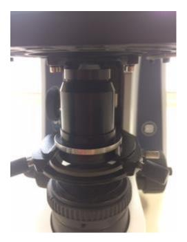
3. Move the condenser up and place the LED light source back into the condenser.
