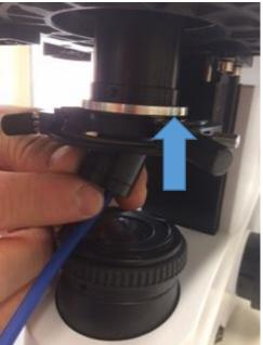
4. Fix LED light source by tightening hexagon screw
