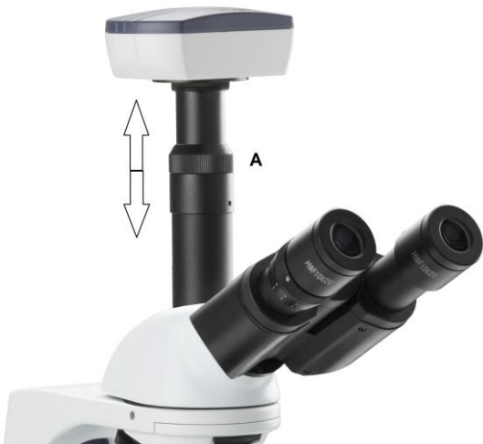
Trinocular bScope head with camera in photo port
