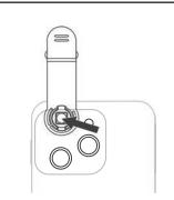
Align the camera of the phone to the center of the circular hole of the adapter clip.
