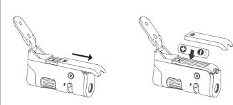
Insert 1 AA alkaline battery and replace battery door.
