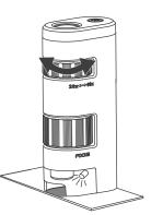
Rotate the focusing ring ⑤ until the image is sharp and clear.
