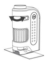
4. Rotate the focusing ring (6) until the image is sharp and clear.
